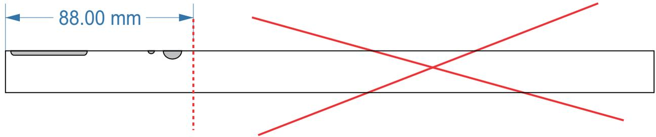
Put your Air Reservoir in to this 88mm tube and align air transfer port holes. After this put inside 88mm tube Crosman 22xx hammer and spring. Also speed adjuster plug which you have included in KIT.
