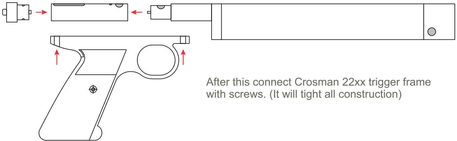
After this connect Crosman 22xx trigger frame with screws. (It will tight all construction)
