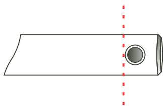
NOTE: to install Crosman 22xx barrel in to Side Lever Breech you must cut barrel exactly after transfer port because now port is already in to breech. Also you will need to turn barrel part which goes in to the breech to 10.96mm diameter
