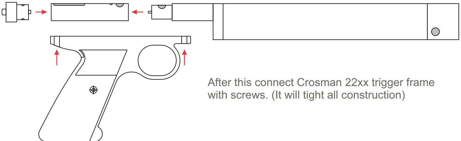
After this connect Crosman 22xx trigger frame with screws. (It will tight all construction)
